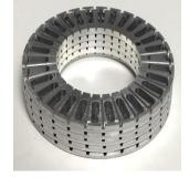
An array of mixing disks 800µm wide mixing areas. A total of 160 areas are in this array. Fabricated with stainless steel.
