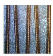
Mixing chip 30µm wide mixing channels with 12µm holes (illuminated from the backside).
