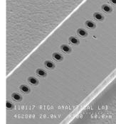
**Through holes** 8µm holes in a device with 150nm pores
