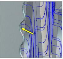
**Ribbed cover plate close-up** Slots in the cover plate create pores when mated to the V channels on the main plate.
