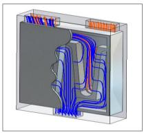
Slotted cover plate An alternate way to create pores is to add slots on the backside of the cover plate.
