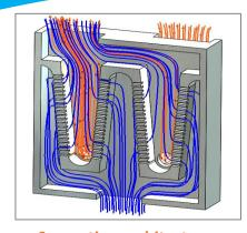
Separation architecture Fluids flow along the surface of a substrate and are separated with pores in the V-shaped walls.
