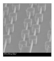
SEM of 80nm pores Isometric view of 60 layers of 80nm pores
